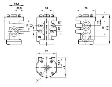
1" valve size, pilot valve Port size: 1"
